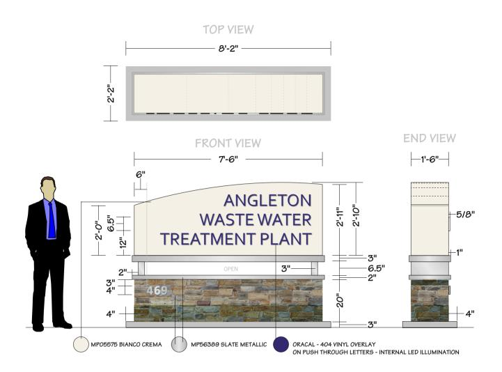
ALL ALUMINUM CONSTRUCTION - INTERNALLY ILLUMINATED BY LEDS WITH PUSH THROUGH ACRYLIC LETTERS & VINYL OVERLAYS (PURPLE) - ROCK INCLUDED \*\* ORIGINAL FONT NAME NEEDED FROM
