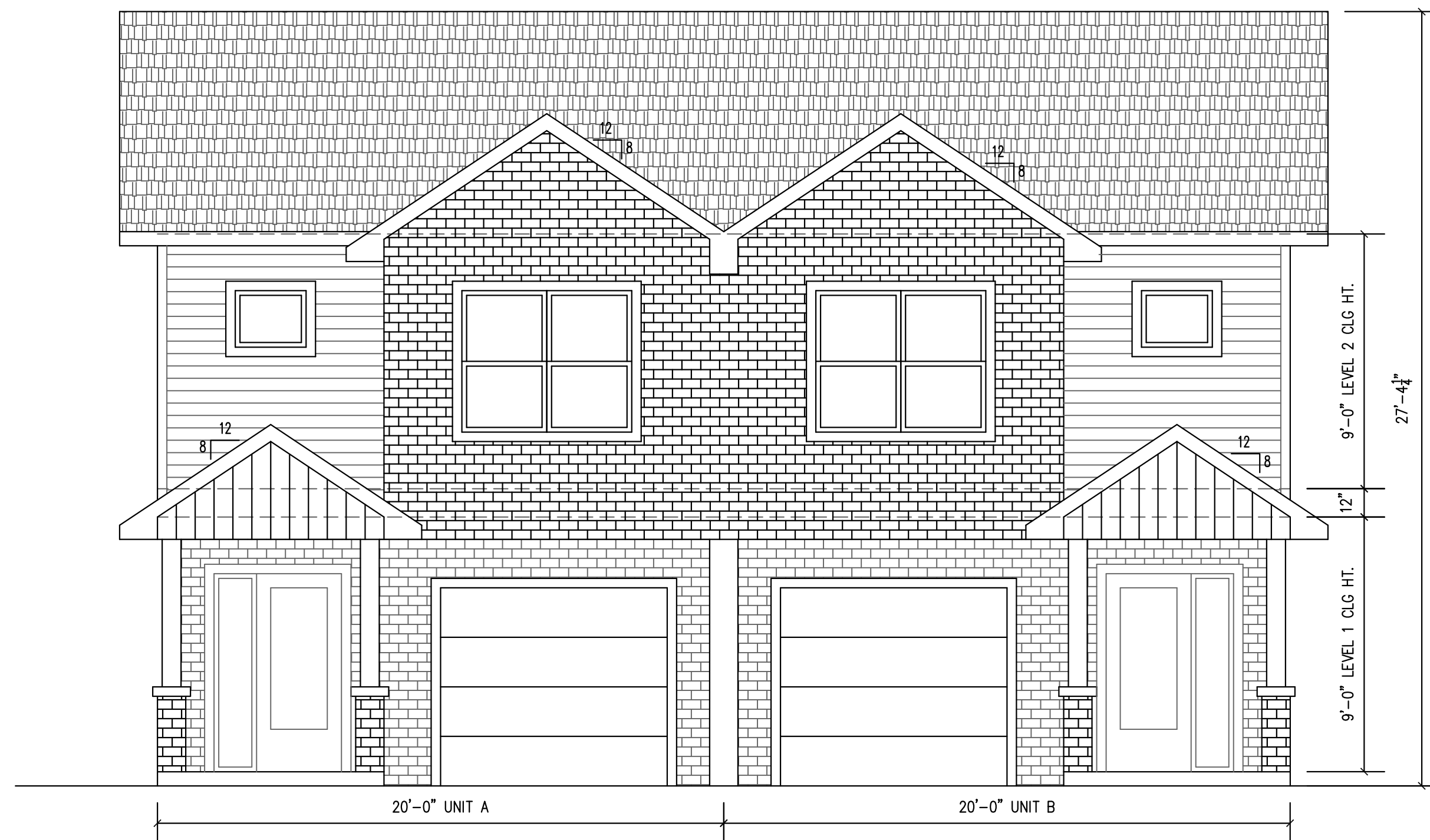
1 EXTERIOR ELEVATION - FRONT VIEW SCALE: 3/8" = 1'-0"
