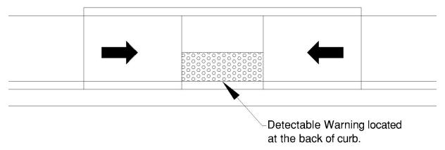
Figure R305.2.2 Parallel Curb Ramps
