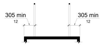
Figure R407.9.1 Extended Ramp Surface
