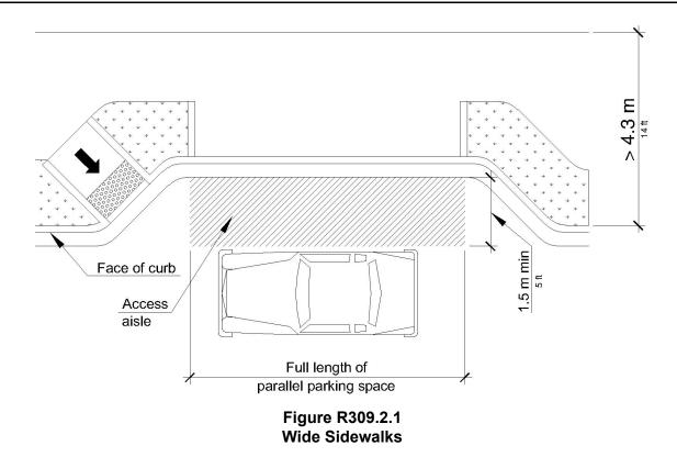
**R309.2.1.1 Alterations.** In alterations where the street or sidewalk adjacent to the parking spaces is not altered, an access aisle shall not be required provided the parking spaces are located at the end of the block face.
