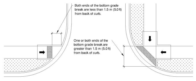
Figure R305.2.1 Perpendicular Curb Ramps
