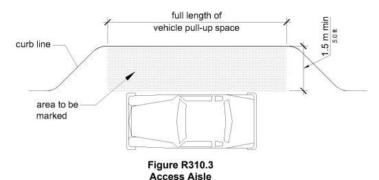
R310.3.1 Width. Access aisles serving vehicle pull-up spaces shall be 1.5 m (5.0 ft) wide minimum.
