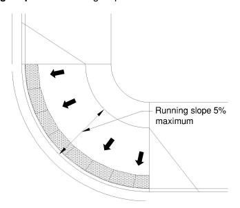
Figure R304.4.1 Running Slope
