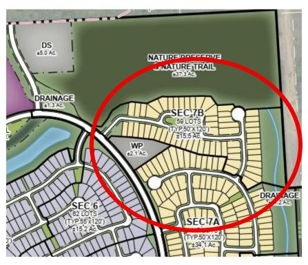
Ashland Development Section 7B Preliminary Plat comprises 26.11 acres, with 59 lots, 4 drainage, landscaping, open space, and utility reserves, and 4 blocks are proposed. The section is located on the northeast section of Sapphire Springs Trail, east of Section 6, and north of Section 7A. (see adjacent Land Plan). The majority of the lots this section in average approximately 50 ft. in width, with only a few 55-ft. lots, at 120' in depth.
