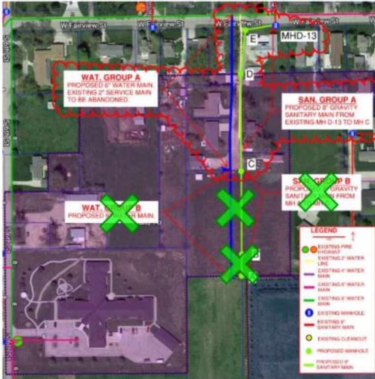
AREA 1-D, GROUP A - Water main and Sanitary Sewer
